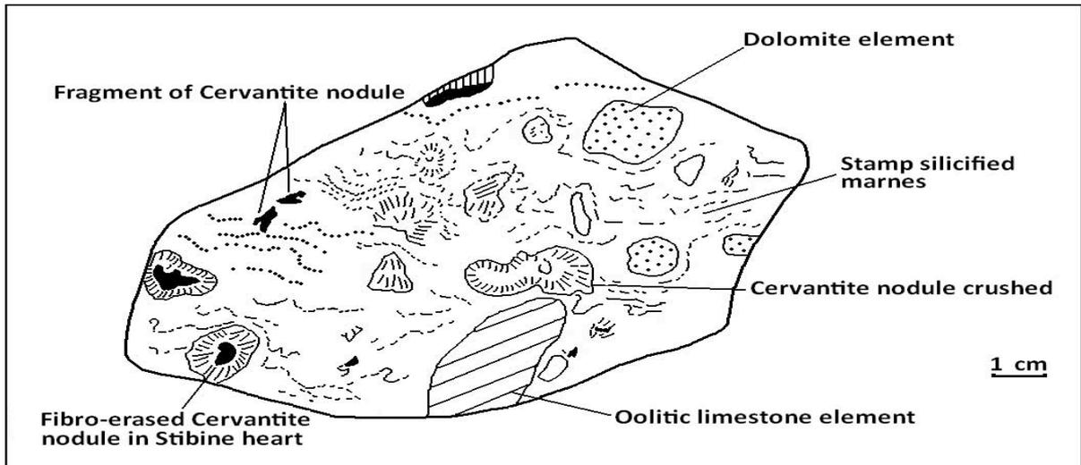
**Figure 3** Sample detail of the ore in the main layer of Portier deposit.
