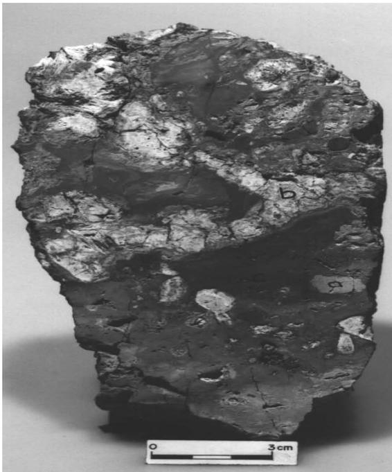
**Figure 4** Sample from the so-called Portier deposit: intra-karstic filling a- Element of dolomite b- stripped cervantite.
