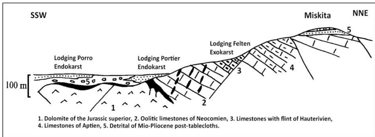
**Figure 2** Geological cross-section through the main deposits of Ain- Kerma.
