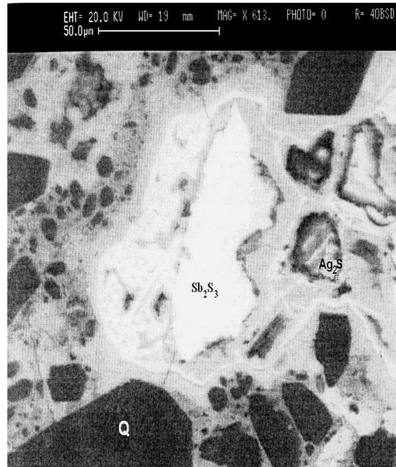
**Figure 5** Photos of retrodiffused electron SEM: stibine ( $Sb_2S_3$ ), quartz (Q), argentite ( $Ag_2S$ ).
