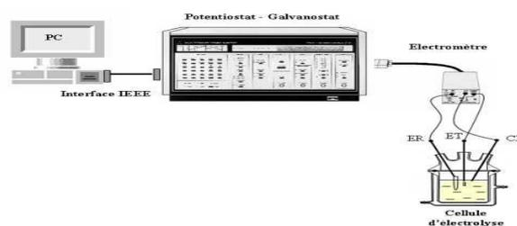
**Figure 1:** Experimental device
