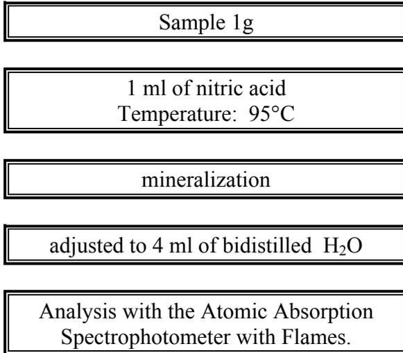
**Figure 3:** Protocol of mineralization according to Amiard *et al.* [1987]
