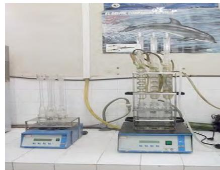
**Figure 2:** Mineralizator (VELP)
