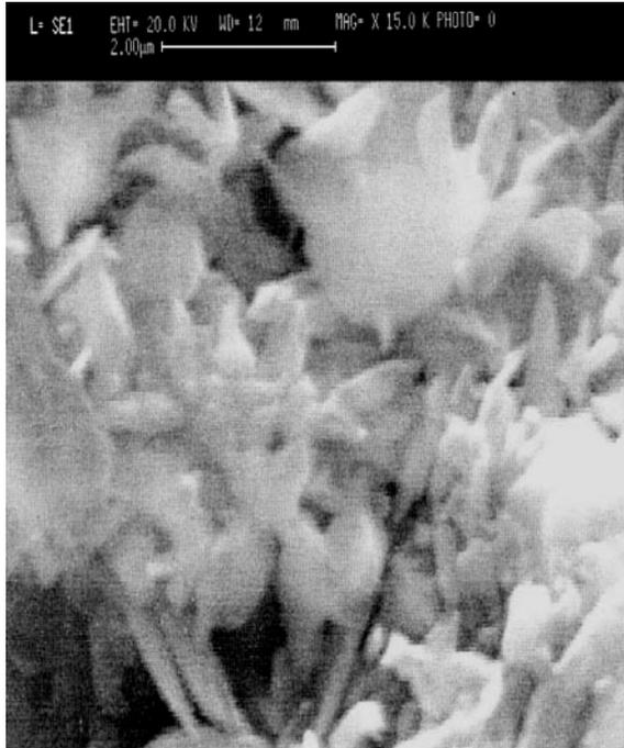
**Figure 6** (SEM). Retro diffused electron image: aspect of twined argentite.
