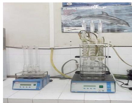
**Figure 2:** Mineralizator (VELP)
