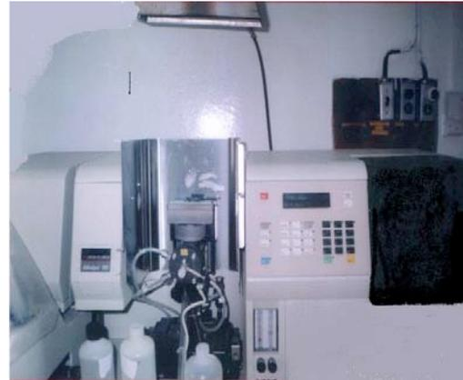
**Figure 4:** The Atomic Absorption Spectrophotometer with Flames
